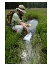
Fiber-optic cable deployed over 1-km length of Wolvorton Meadow stream; ice is for calibration
