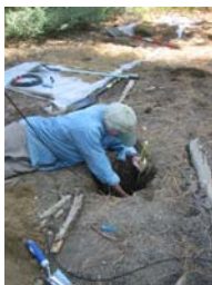
Installing Echo probes for soil moisture & temperature
